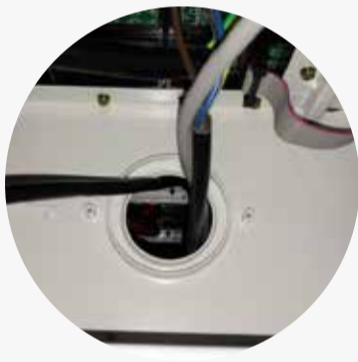
Data cable and power cable goes inside the cabinet via cabinet up and down holes
