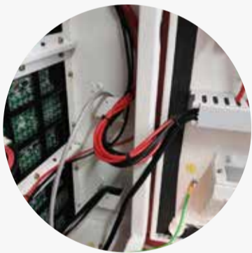
Data cable and power cable goes inside the cabinet via the cabinet side hole
